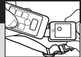
Remove receiver from charger. Light will flash yellow. Press button on transmitter within 30 seconds. The components now work together.
