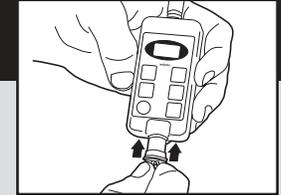
Charge the collar 12-14 hours. Be sure to cover the charge jack with the gray plug when done. Insert batteries in the transmitter positive (+) side out.
